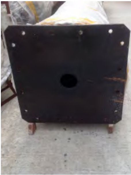
Base-Plate showing Bolt-holes
